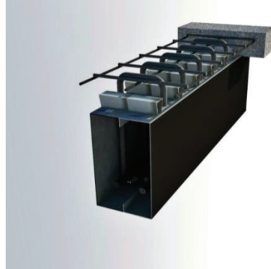
FIGURE 2. CFS Composite beam design with box section
