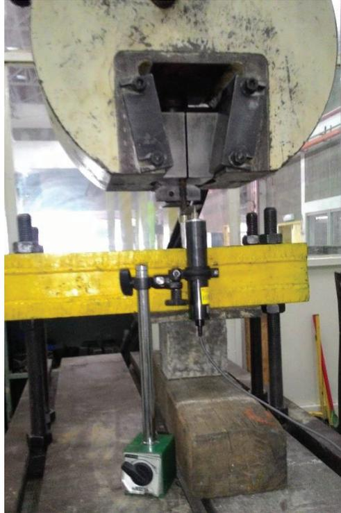
FIGURE 1. Experimentation setup for direct tension pull-out test
