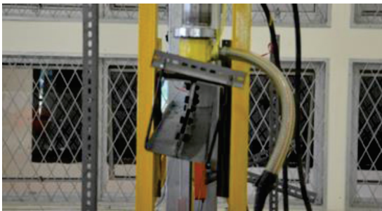
a) Failure mode on structure (torsional buckling)
