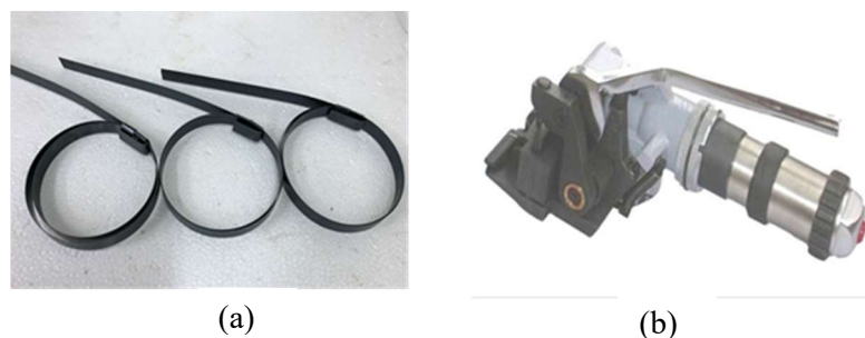
Figure 3. Steel straps and the tensioner (a) Steel straps hoops (b) Pneumatic tensioner.
