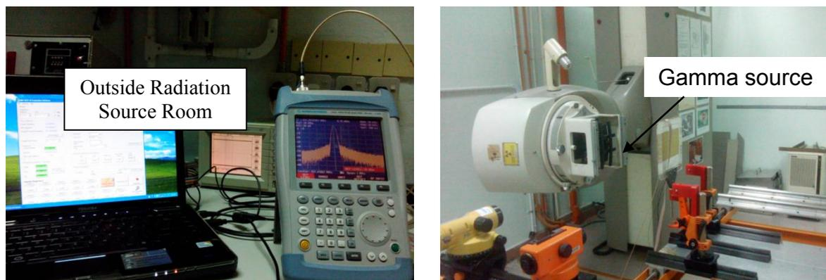
Figure 3: Radiation test setup at Malaysia Nuclear Agency
