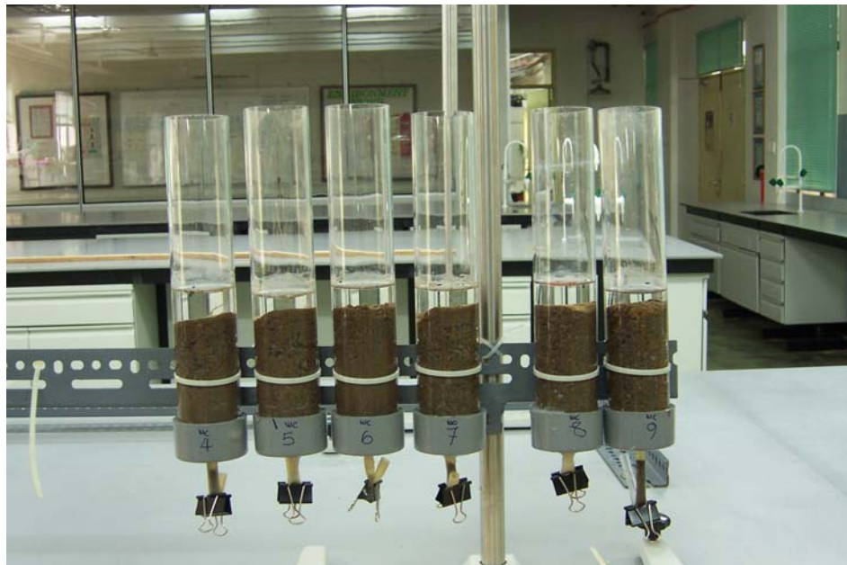
Figure 4 Experimental setup of leachability column test
