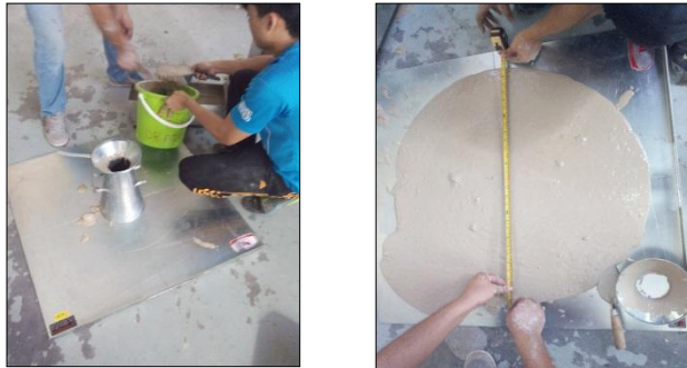
Fig 1. Procedure for Slump-Flow Test.
