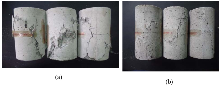
Figure 4. Mode of failure for (a) Normal Concrete (NC) and (b) Treated Crumb Rubber Steel Fiber Concrete (TCRSFC).
