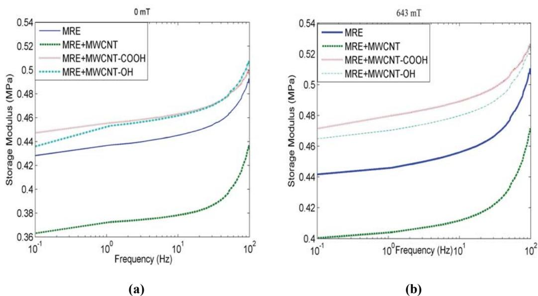
**Figure 1** Storage modulus vs frequency (a) 0 mT (b) 643 mT
