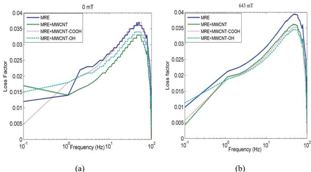
**Figure 2** Loss factor vs frequency (a) 0 mT (b) 643 mT
