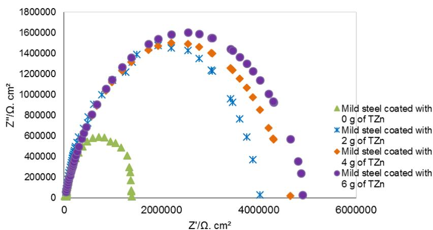
**Figure 3.** Nyquist plots of steel coated with absence and presence of TZn.
