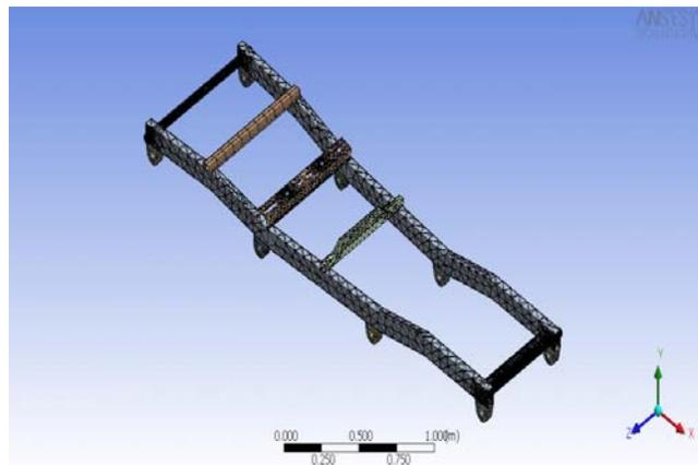
Figure 4.18: Truck chassis model meshed with tetrahedral -10 elements
