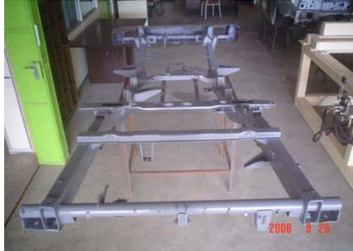
Figure 4.4: Ladder type structure
