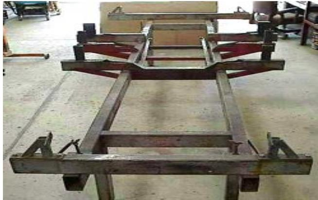
Figure 4.1: The main structures of ladder-type chassis
