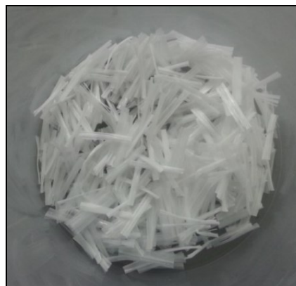
Fig. 2. Polypropylene fibre – fibrillated
