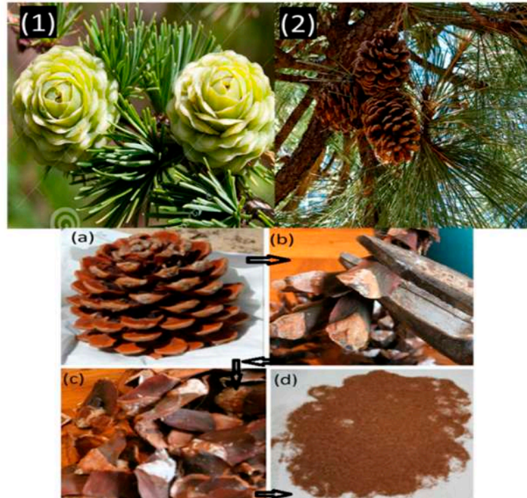
Figure 1. Pine cone flowers in their natural state (1,2) and extraction of pine cone fibres (a–d).
