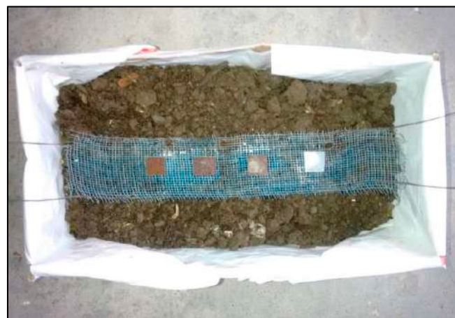
Figure 5. Compost box with samples placed inside.
