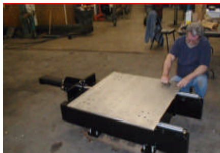
Figure 1.1: Electric shaking table [1]
