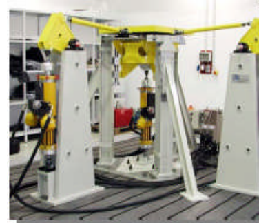
Figure 1.4: 6 DOF shaking system [3] Figure 1.5: 3 DOF shaking system [3]
