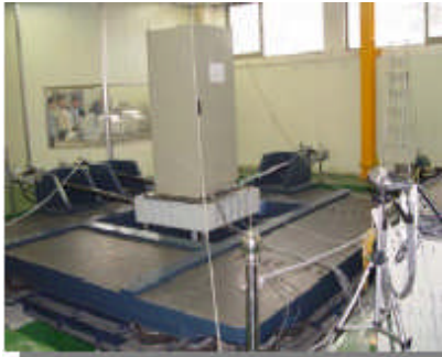
Figure 1.4: 6 DOF shaking system [3] Figure 1.5: 3 DOF shaking system [3]
