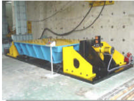
Figure 1.6: 1 DOF shaking system [3]
