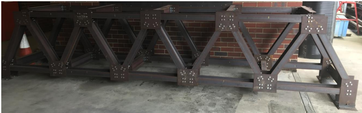
Fig. 2 - Laboratory scaled steel truss bridge structure
