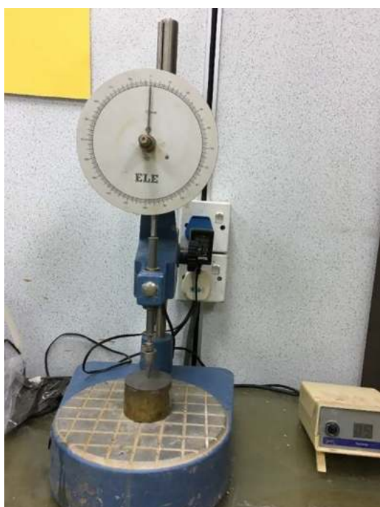
Fig. 6. Liquid limit sample and apparatus.
