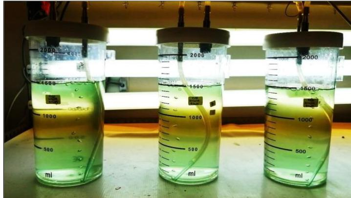
**Figure 1.** The 2 L photobioreactor used in the cultivating microalgae to optimise the biomass production of *A. platensis* under specific conditions.
