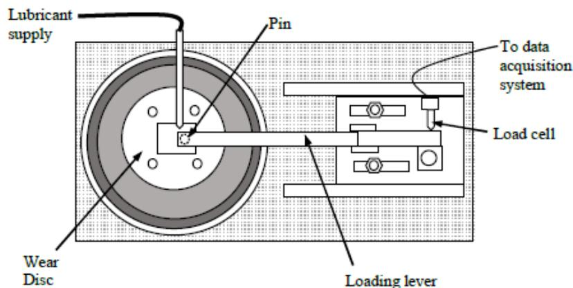
**Figure 2.** Pin-on-disc friction tester (Hamdan et al., 2018)
