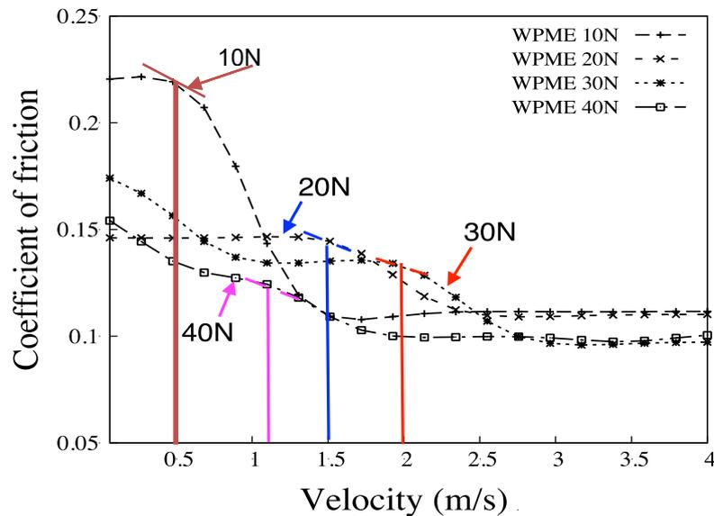
**Figure 3.** Coefficient of Friction (CoF) measured for WPME at varying velocities with different loads for tested lubricants
