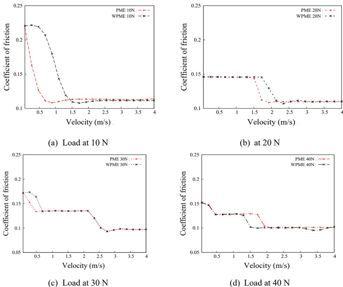
**Figure 4.** Stribeck curve measured for (a) WPME and (b) PME with different loads analysis.
