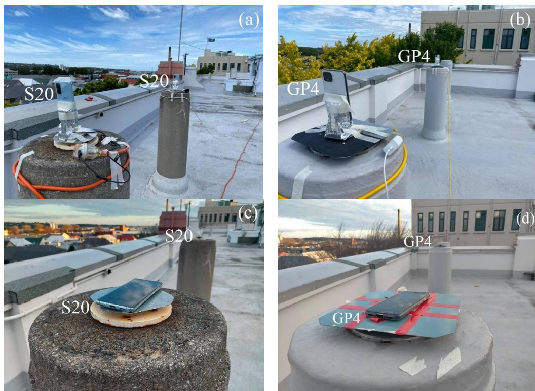
Figure 4. Short-baseline setup configurations with smartphones internal antennas in upright (a,b) and lying down (c,d) positions.
