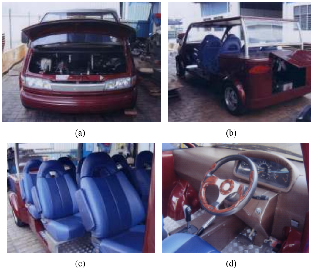
Figure 1.1: The tramcar as viewed from various angles; (a) the front view of the tramcar, (b) the rear view of the tramcar, (c) the passenger seating in the tramcar, and (d) the interior view of the driver's compartment
