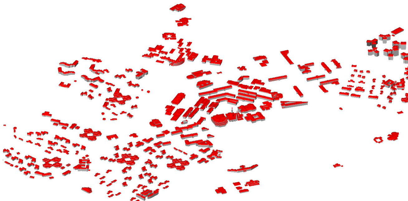
Figure 12. Virtual 3D of Universiti Teknologi Malaysia campus with 381 buildings as displayed using FZK Viewer.
