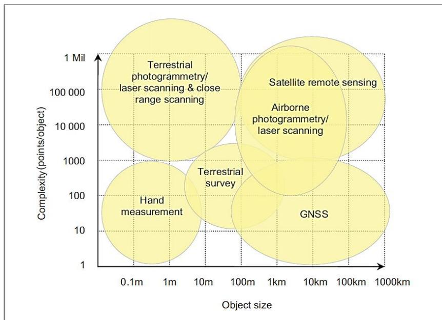
Figure 1.1 3D survey systems categorised by object size vs probing density of points for detection (scale) adopted from (Barber, 2011a)
