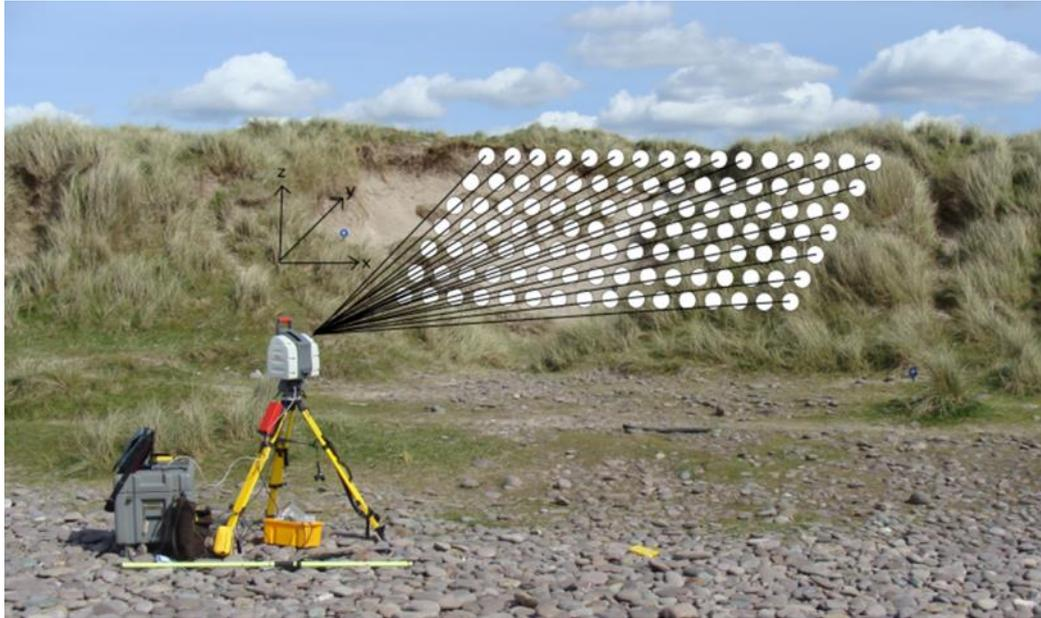
Figure 1.3 Geodetic TLS – Surface points represents the location of laser reflection (Kandrot, 2013)
