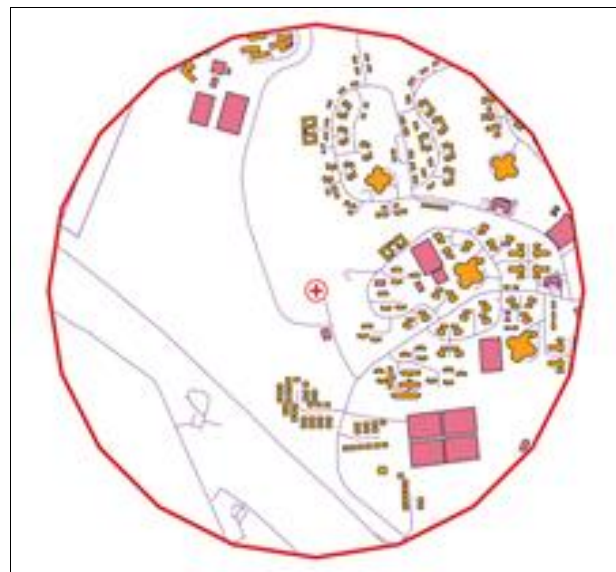
Figure 2. Example of buffer analysis (distance to UTM Health Centre)
