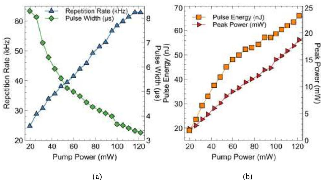
**Figure 3.** Relationship between (a) repetition rate and pulse width, and (b) pulse energy and instantaneous peak power at different pump power.
