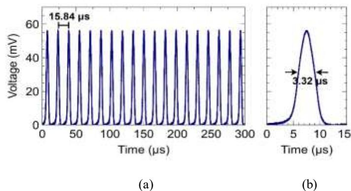
**Figure 2.** (a) Typical pulse train and pulse width at pump power of 121.5 mW and (b) the pulse-to-pulse separation in  $15.84 \mu\text{s}$  with single pulse width of  $3.32 \mu\text{s}$ .
