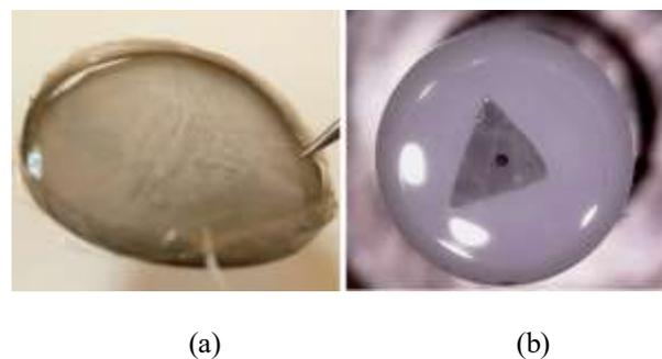
**Figure 1.** Physical image of AgNP-PVA SA after 3 days drying under room temperature and (b) transferred onto a FC/PC fibre end.
