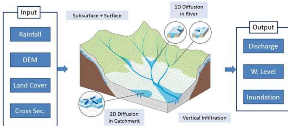
**Figure 2.** Schematic diagram of Rainfall-Runoff-Inundation (RRI) Model.
