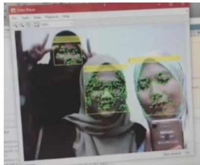
Figure 6. Example of image processing result: Face Detection.
