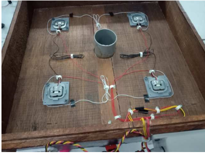
Fig. 3. SGLC sensors installed on top of supporting platform
