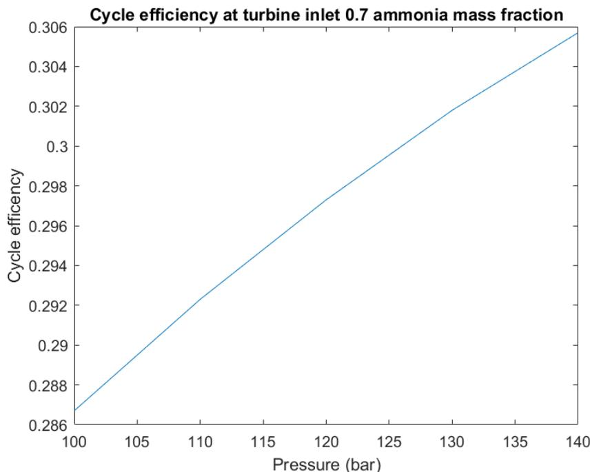
Figure 3. Effects of turbine inlet pressure on Kalina cycle efficiency
