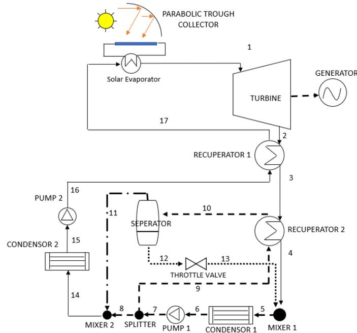
Figure 1. The Kalina cycle KC-12 layout [adapted from (Modi et al. 2016)]
