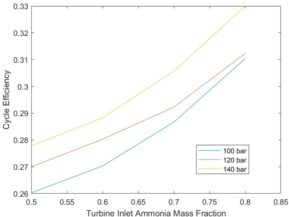
Figure 4. Effects of turbine inlet ammonia fraction on cycle efficiency at different inlet turbine pressures
