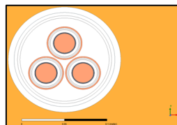
Figure 4 3*185 mm 2 triangular 11 kV cable
