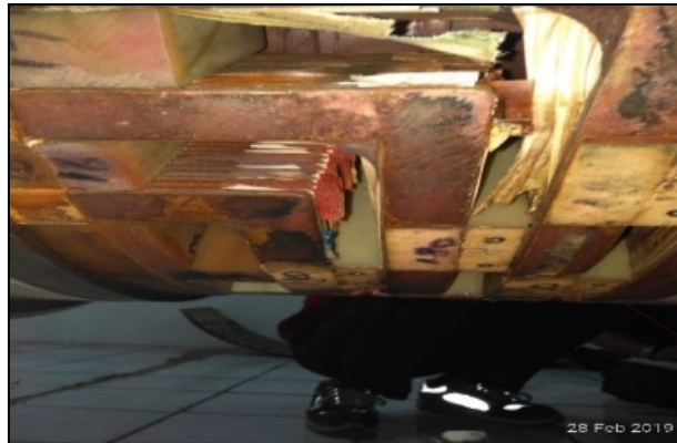
Figure 6. Migration insulation interturn elbow end winding area.
