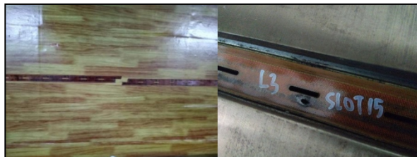
Figure 7. Degradation insulation interturn slot coil.
