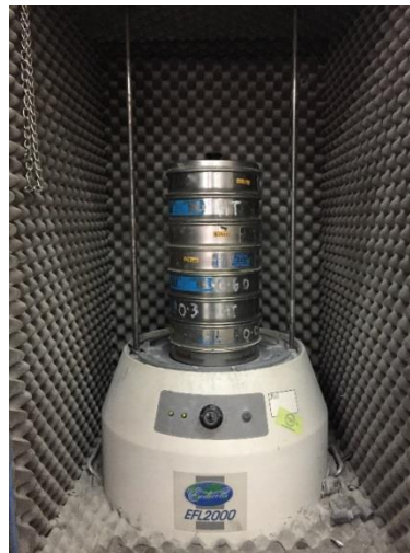
Figure 2. Mechanical Sieve Shaker and Test Sieves
