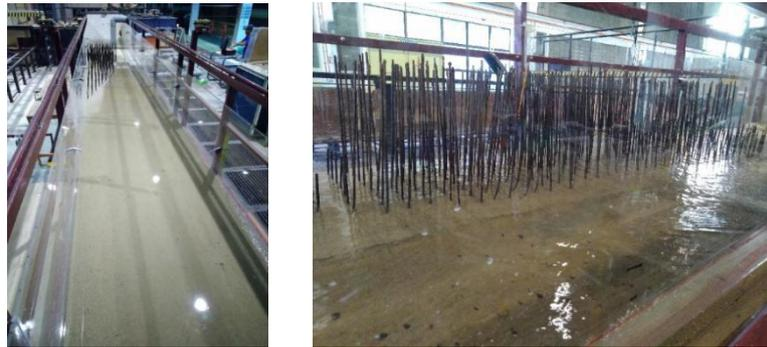
**Figure 3.** The condition of cylindrical rods installed in the channel as vegetation.
