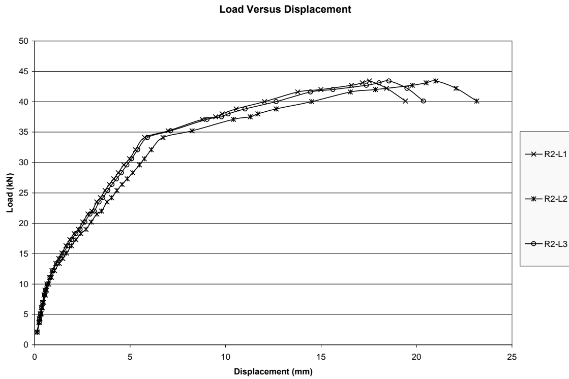
Figure 4.33: Load-displacement curve of RC-GFRP beam.
