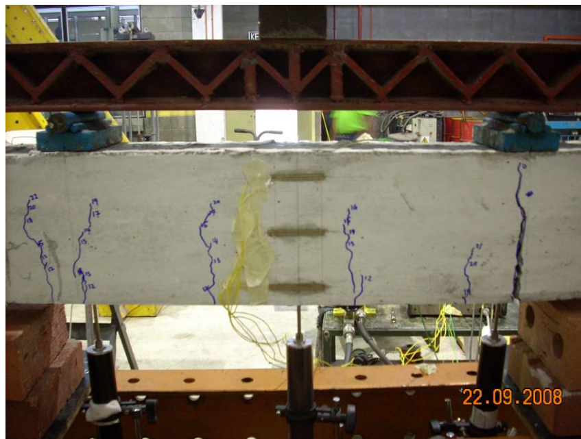
Figure 4.30: Flexural cracks were observed in control beam.
