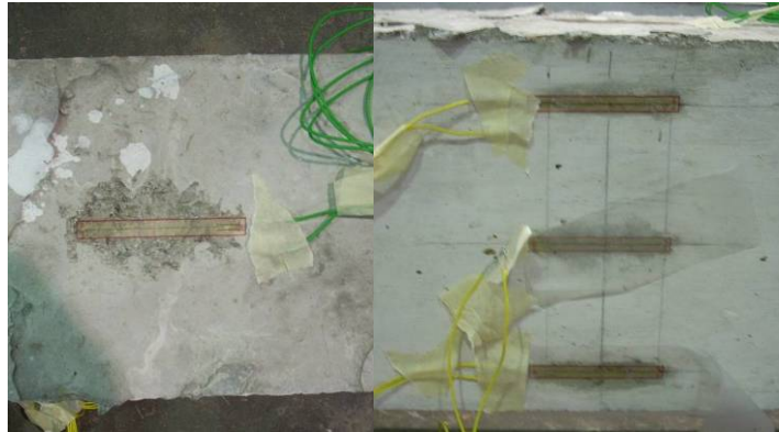
Figure 3.25: Four strain gauge are installed at top of the beam and side beam.
