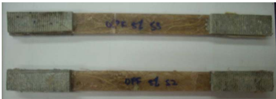
Figure 3.16: Straight sided specimen size of oil palm fibre composite.
