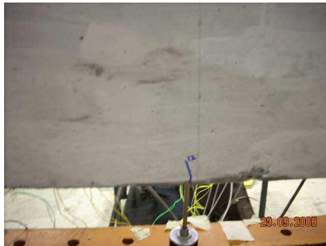
Figure 4.34: Initial crack was found at 12kN of applied load in GFRP-RC beam.
