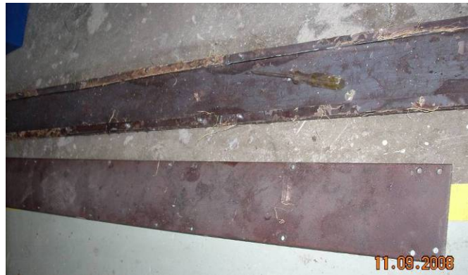
Figure 3.23: Steel mould is made to fabricate composite plate
