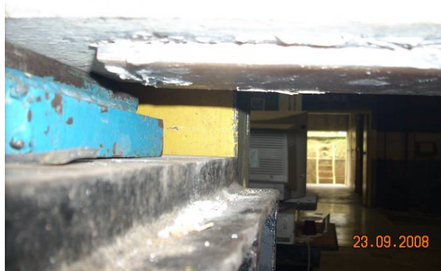
Figure 4.36: GFRP plate end interfacial debonding was observed after ultimate load.
