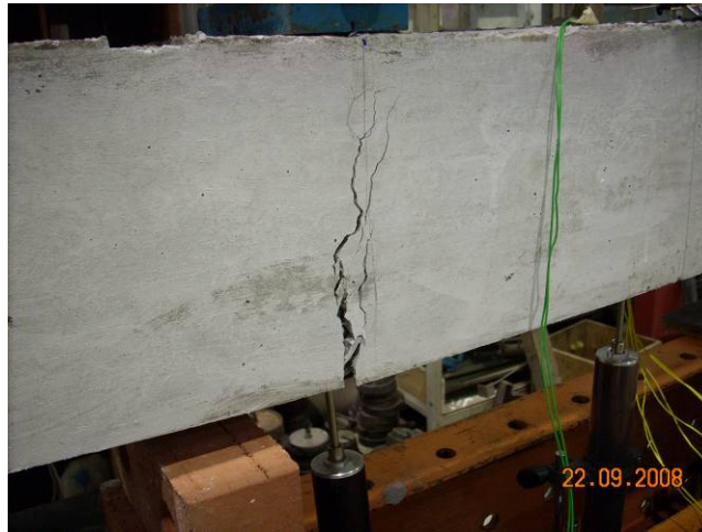
Figure 4.29: Large flexural crack was found under the applied load after the control beam failed.
