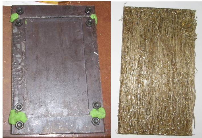
Figure 3.9: Open steel mould is made and the product of open-mould system.
