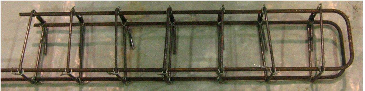
Figure 3.20: Shear link and anchorage bar.
