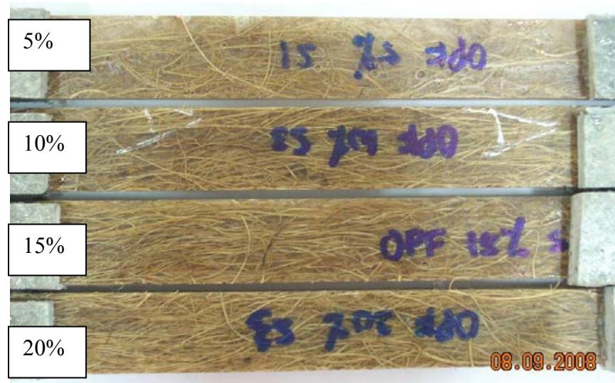
Figure 4.11: The appearance of different fibre volume fraction composite.
