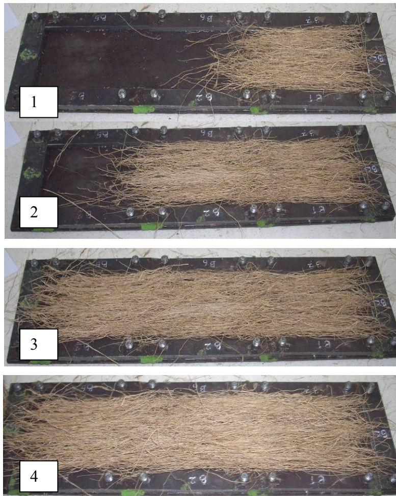
Figure 3.12: The sequence of laying the fibres before composite is fabricated.
