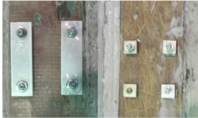
Figure 3.26: Dummy plates PIF-11 are used when mounting the PIF-21 jig to the composite plate.
