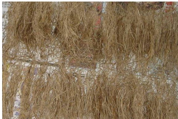
Figure 3.3: Processed oil palm fibres after combing process.
