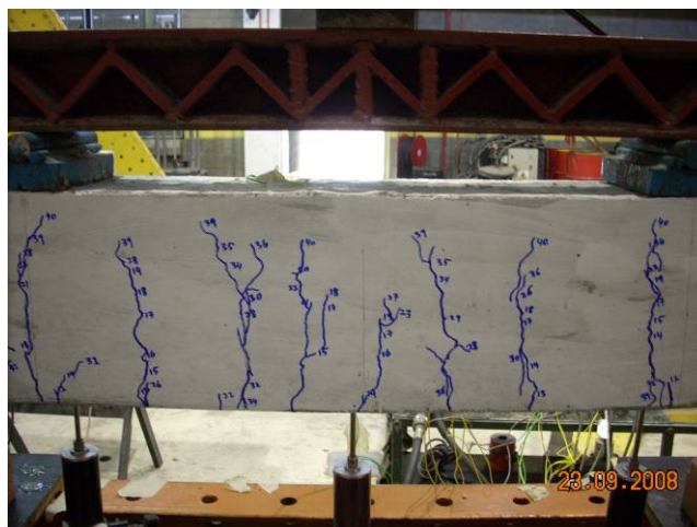
Figure 4.35: Flexural cracks were observed in GFRP-RC beam.
