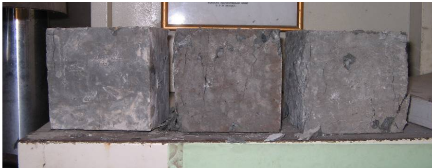
Figure 4.27: Longitudinal cracks were found on tested concrete cubes at 28 days.
