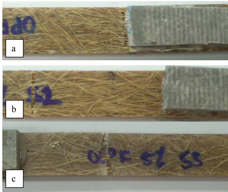
Figure 4.16: Typical failure pattern of unidirectional composites under longitudinal tension, a) fracture near tab, b) and c) fracture in gage length.
