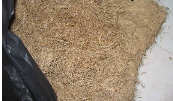
Figure 3.2: Oil palm fibres is obtained in a rectangular bales. The Fibres are curly, different direction and entangled.
