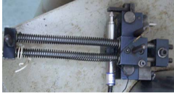
Figure 3.17: Extensometer with 50 mm gage length.
