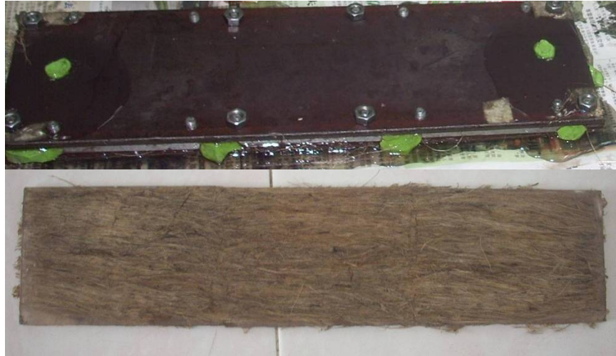
Figure 3.10: A close-mould system and the product of close-mould natural fibre composite.
