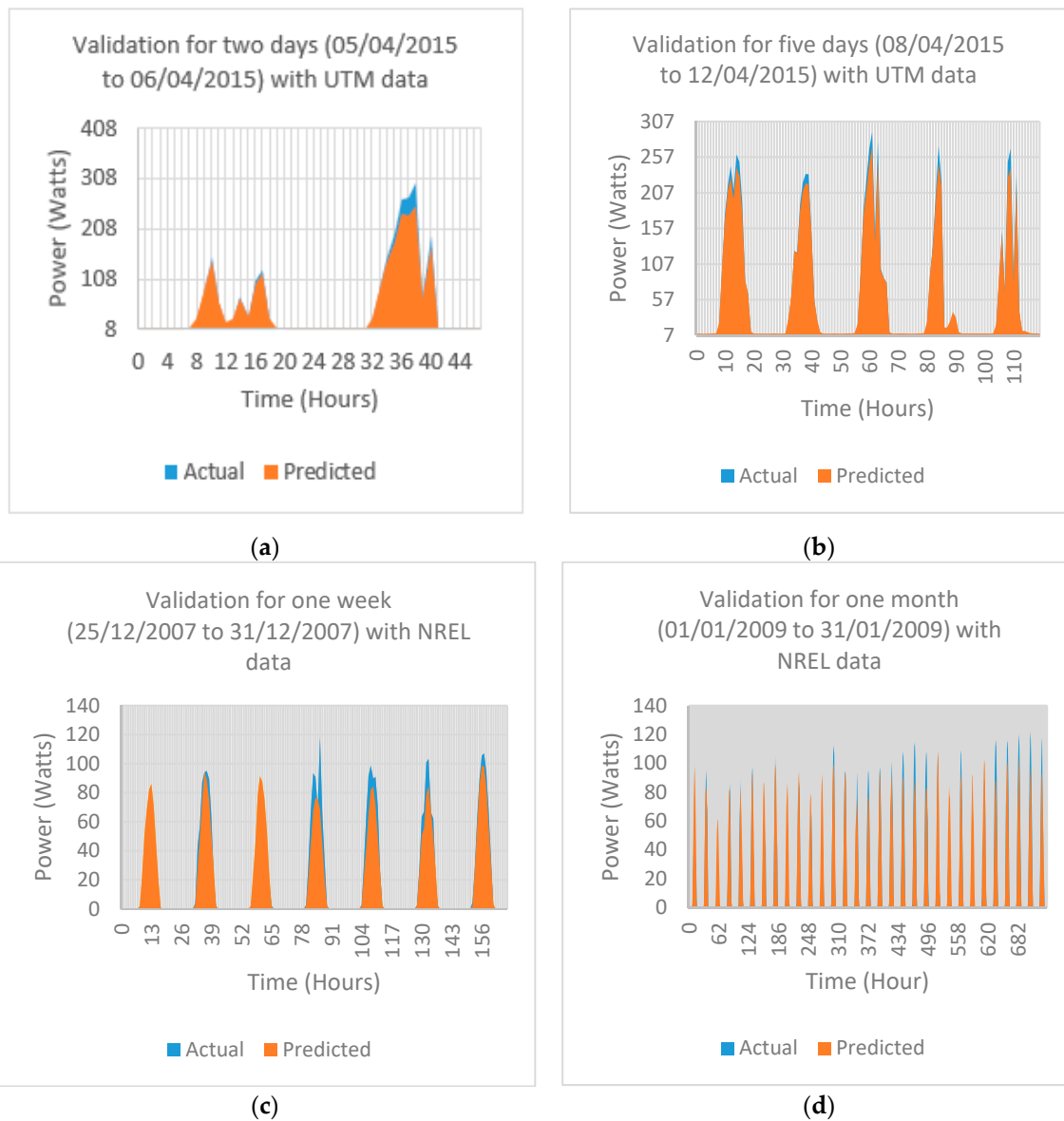
Figure 10. (a,b) show comparison between actual and predicted PV power for validation with UTM Malaysian data; (c,d) show comparison between actual and predicted PV power for validation with NREL USA data.
