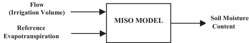
Fig. 3 – Multiple Input Single Output (MISO) model based on the hydrological balance.
