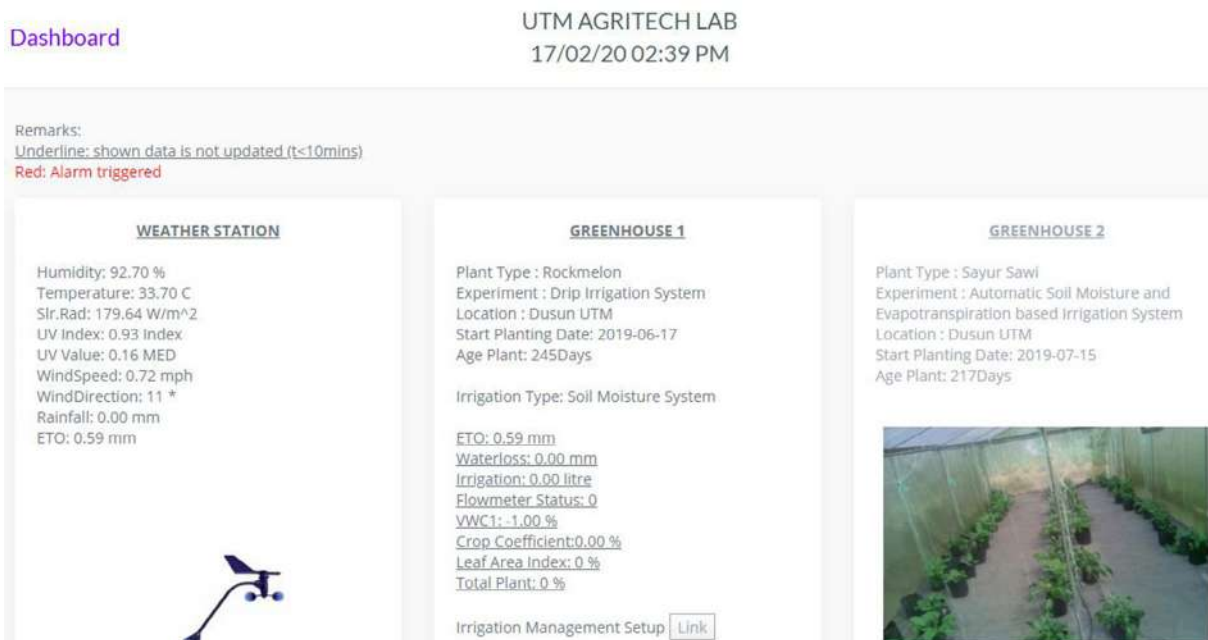
Fig. 2 – UTM AgriIoT Dashboard for Monitoring [77].
