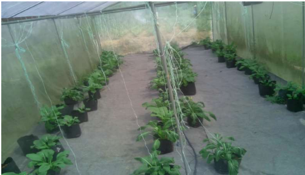
Fig. 10 – Experimental setup of smart drip irrigation system for Mustard Leaf cultivation in a greenhouse monitored via IoT based Raspberry Pi camera.
