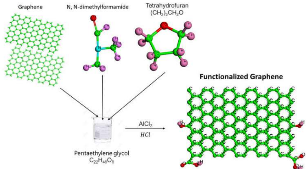
Figure 1. Schematic illustration of the covalent functionalization of graphene.
