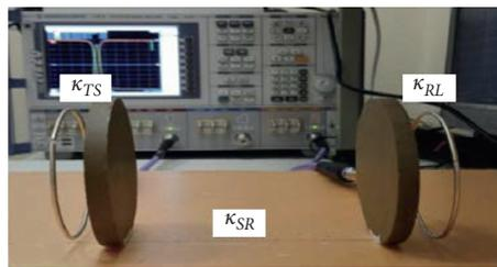
FIGURE 12: Design of the WPT system as in [46, 47].
