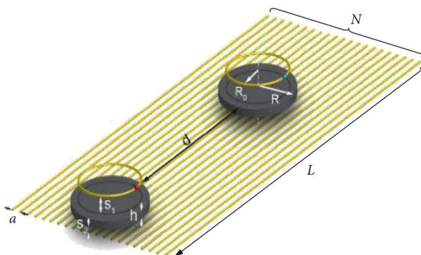
FIGURE 14: Design of the WPT system as in [34].
