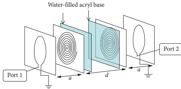
FIGURE 10: Design of the WPT system as in [43].
