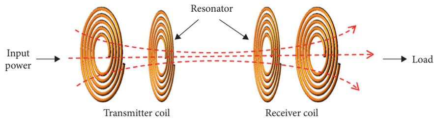
FIGURE 2: Basic block diagram of the MRC system.
