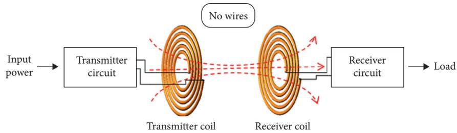
FIGURE 1: Basic block diagram of WPT.
