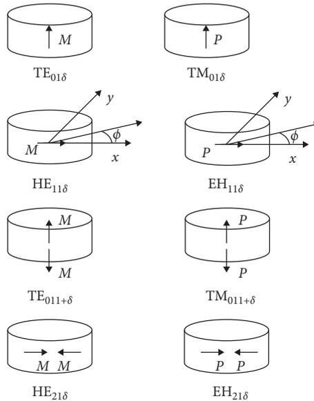
FIGURE 6: Nature of radiation for different modes of the cylindrical dielectric resonator.  $M$  is magnetic dipole and  $P$  is electric dipole [40].
