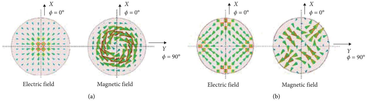
FIGURE 7: View of the electric and magnetic field intensity using HFSS eigenmode method. (a)  $TM_{01\delta}$ ; (b)  $HEM_{21\delta}$  modes [41].
