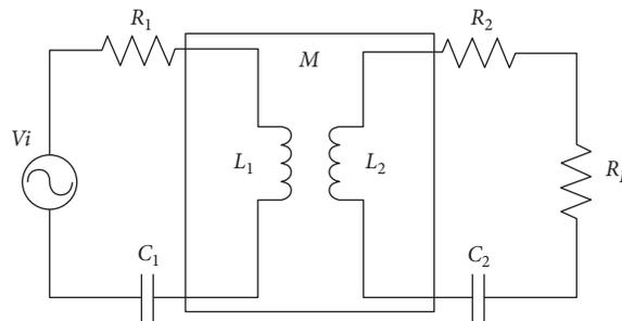
FIGURE 3: Circuit topology of the MRC system.
