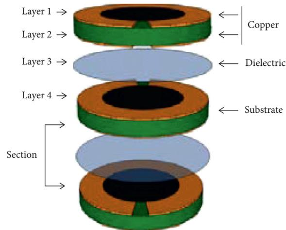
FIGURE 17: Design of the WPT system as in [54].
