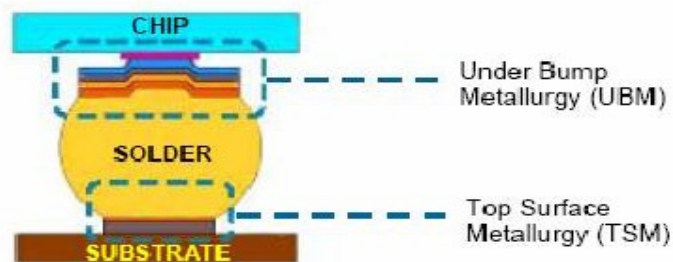
Figure 2.12 Solder Bump Structure
