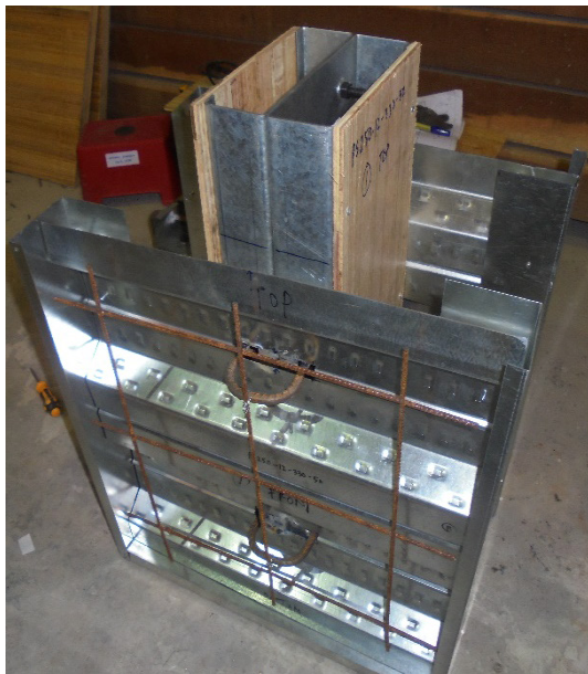
(a) The profiled metal decking slabs
