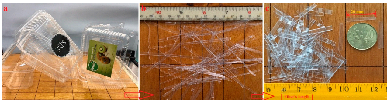
Figure 3. Preparation of waste plastic food tray (WPFT) fibres: (a) waste plastic food tray; (b) plastic strips; (c) fabricated fibres.
