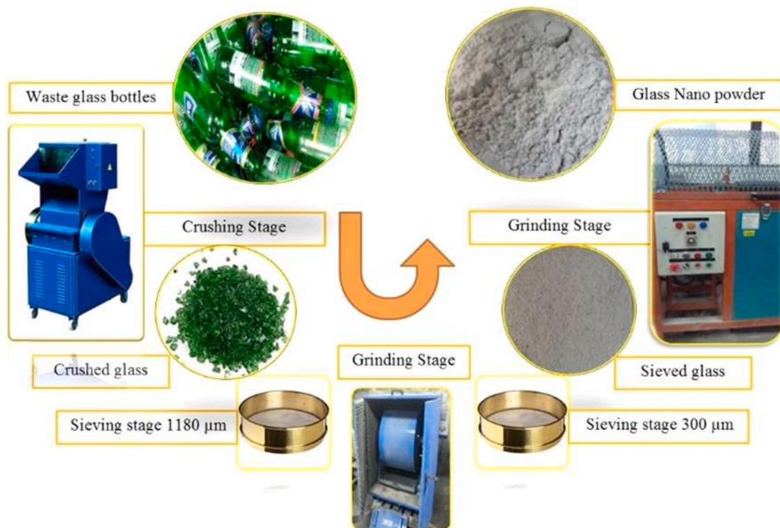
Fig. 1. Preparation stages of WGBNP.
