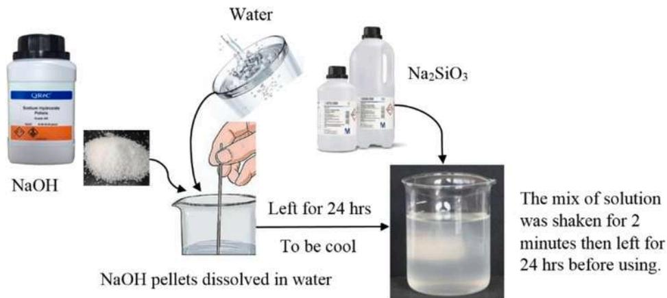
Fig. 2. Procedure for the alkaline activator solution preparation.
