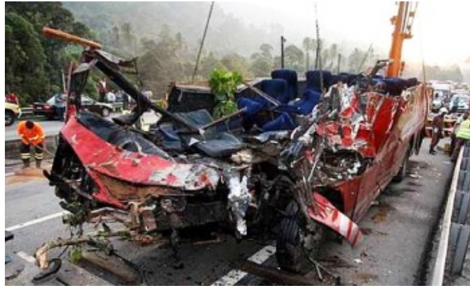
Figure 1.8: The severe damage of bus after rollover accident (Courtesy of www.thestar.com.my ).
