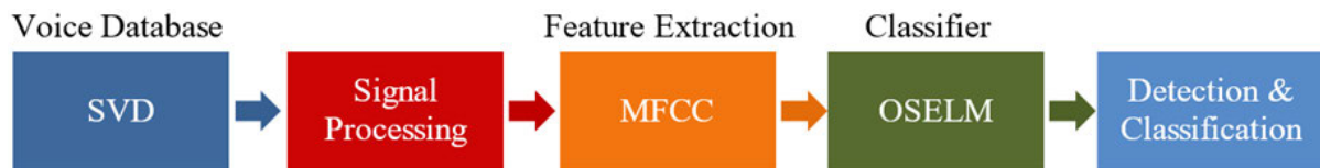
FIGURE 1. Flowchart of the proposed system in voice pathology detection and classification.
