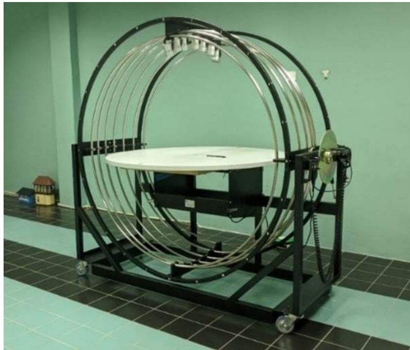
Fig. 2. The sun-emulator heliodon model at the Faculty of Built Environment, UTM Johor Bahru.
