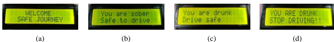
Figure 5. LCD display during, (a) System start up, (b) Sober, (c) Mildly drunk, and (d) Drunk
