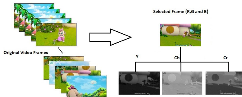
Figure 3. Original video frame RGB to Y, Cb and Cr color space
