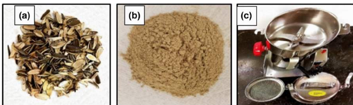
Figure 3. (a) Black sunflower shell raw waste converted into (b) powdered form using (c) a food processor [51].
