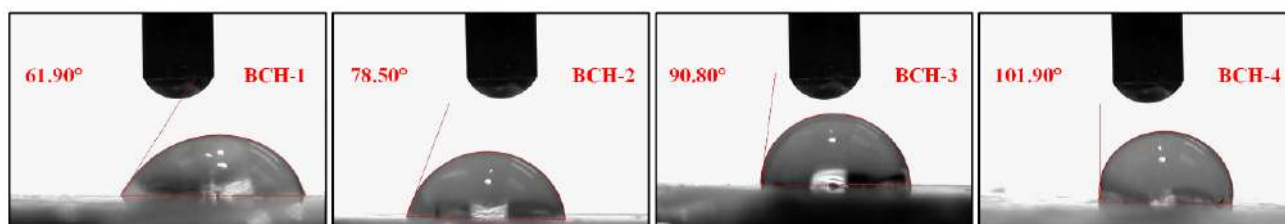
Figure 4. The measurement of water contact angles at different time intervals to determine the hydrophilicity of hydrophobicity of hydrogels with an increasing amount of rGO and time ( t = 5 s).
