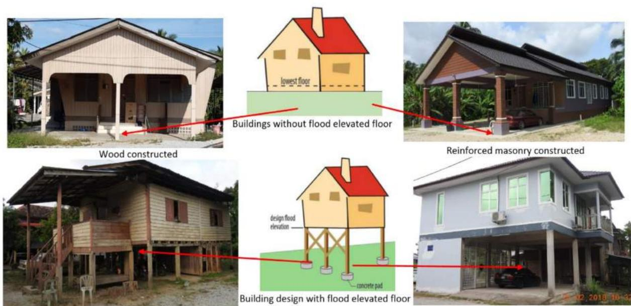
**Figure 13.** An illustration of elevated and non-elevated buildings.
