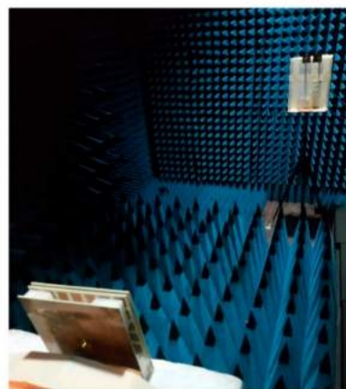
Figure 9. Simulation vs. measurement results of monostatic RCS suppression presented at different frequency points. (a) VP wave incidence. (b) HP wave incidence. (c) Measurement setup.
